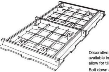
Decorative Edge in Brass or Stainless Steel is available in heights of 18mm, 50mm and 75mm to allow for tiling, paving etc.
